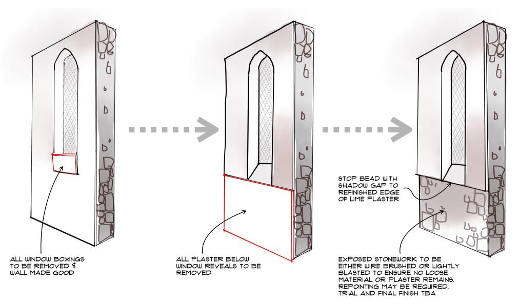
GENERALLY - REMOVE **ALL** LOOSE/ SPRUNG PLASTER, PATCH REPAIR WITH LIME PLASTER \$ REDECORATE
